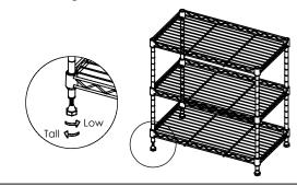
Please make sure that you have the Wire Shelf(A) the correct way up. Hold the shelf and slide the top of four lower poles through the bottom of each shelf at its corners until there is snug fit.
