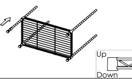
Refer to the Step (3) to assemble the final shelf. And then push Cap(E) on top end of Upright pole(B).
