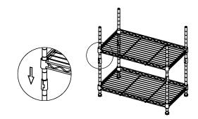
Pushing firmly down on every wire shelves at corners by rubber mallet to ensure all the shelves in a place over the plastic clips. And screw leveling feet in or out to attain proper leveling.
